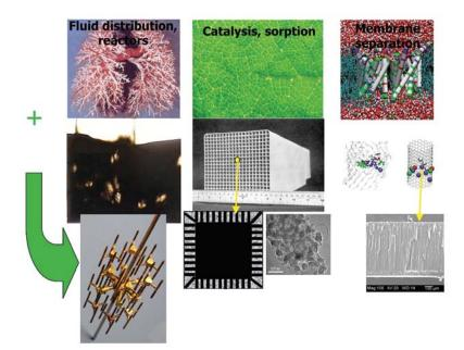
**Figure 1:** Multiscale nature-inspired chemical engineering. Left: fractal fluid distributors for multiphase reactors, inspired by the structure of the lungs and vascular network. Middle: design of hierarchical catalyst pore networks, inspired by the venal architecture of leaves. Right: design of membranes for high-flux highly selective separations, inspired by protein channels in cell membranes.
