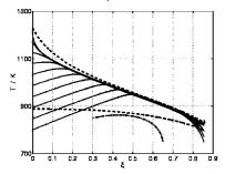
**Picture 6.** The highway in state space for chemical reactors defined by temperature and composition along the black band. Reprinted with permission of *Chem. Eng. Sci.*
